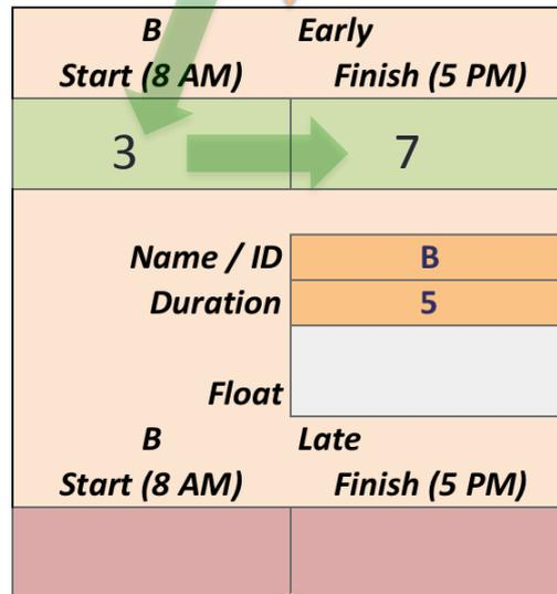
We will calculate all Early Start and Finish Times in a "Forward Pass", and then do a "Backward Pass" to calculate all the Late Start and Finish times
